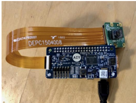
Fig. 5. Cable flex is turned around.
