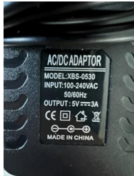
Fig. 7. The power source is enough.
