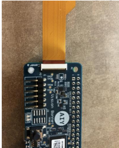
Fig. 2. Cable is not properly secured to the latch.
