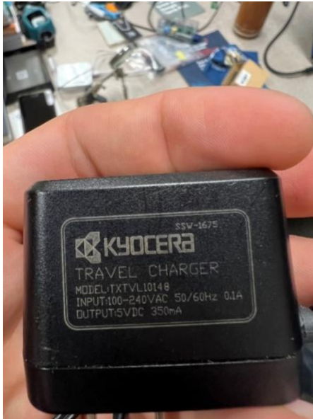
Fig. 6. The power source is not enough.
