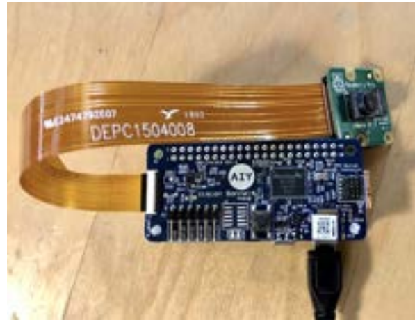
Fig. 5. Cable flex is turned around.
