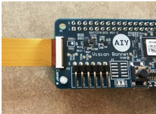
Fig. 2. Cable is not properly secured to the latch.
