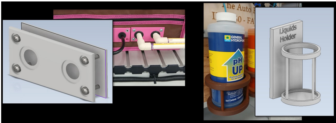
Fig. 10. To effectively seal the plumbing penetrations into the grow tent, custom flanges were designed and printed from matching filament (a). The pH and plant food container mounts were customized for the container sizes and fabricated to mount to the outside of the hydroponics platform (b).
