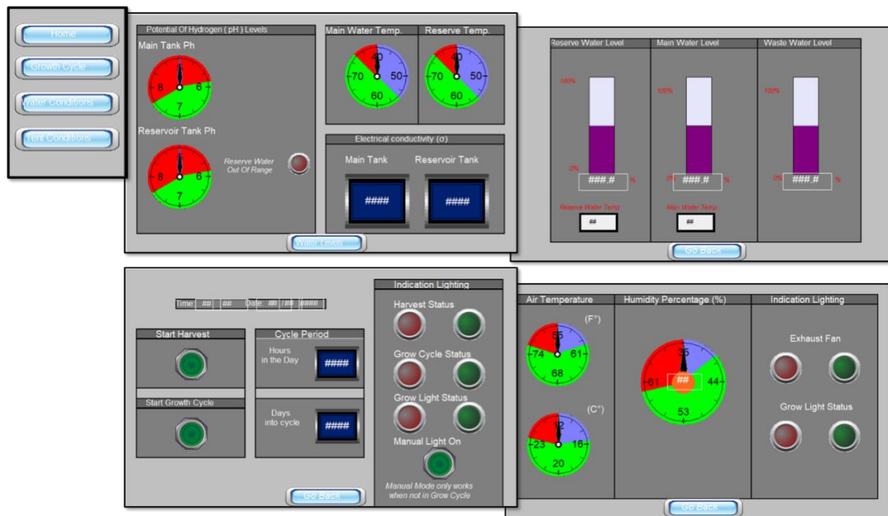
Fig. 8. HMI control of the hydroponics system requires the ability to monitor and control many different variables at once. Pages and submenus were leveraged to provide the operator with concise access to everything.
