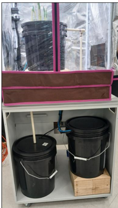
Fig. 4. Completely enclosed grow tent housing the main tank, plants, humidifier, exhaust fan, and lighting. The tent can be closed to outside light during the growing phase. Any penetrations into or out of the grow tent are sealed to create a controlled microclimate.
