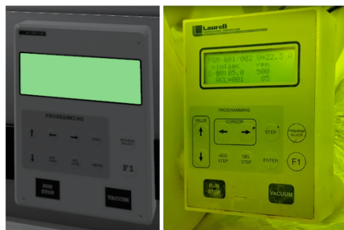
Fig. 3. The digital spinner controller (left) compared with the real controller (right)
