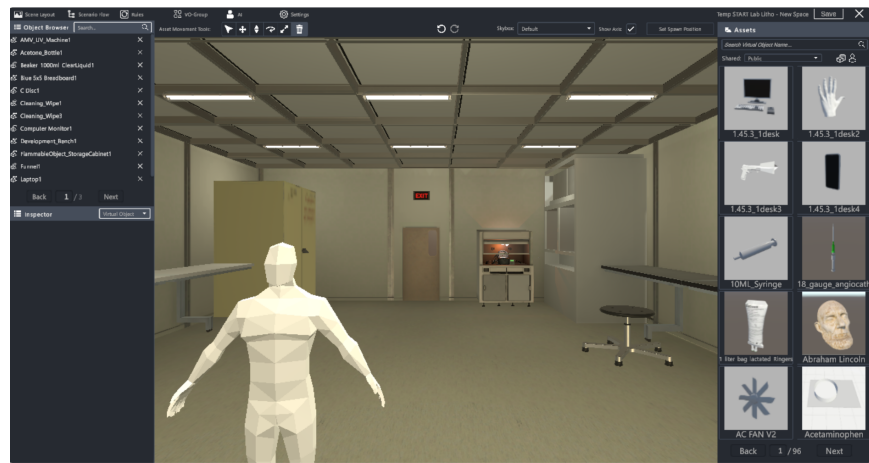
Fig. 4. Screenshot of the Scene Layout tab used to develop the simulation. The catalog on the right shows assets from the library that can be dragged into the simulation.
